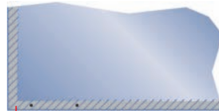
3 Insulating glass: coating acts as an invisible alarm loop and is monitored by an evaluation unit
